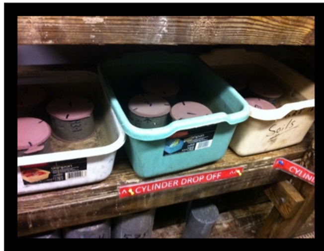
Figure 2.3 (Left): Picture of a cylinder getting removed from the mold Figure 2.4 (Right): Picture of cylinders submerged in water prior to compressive strength testing
