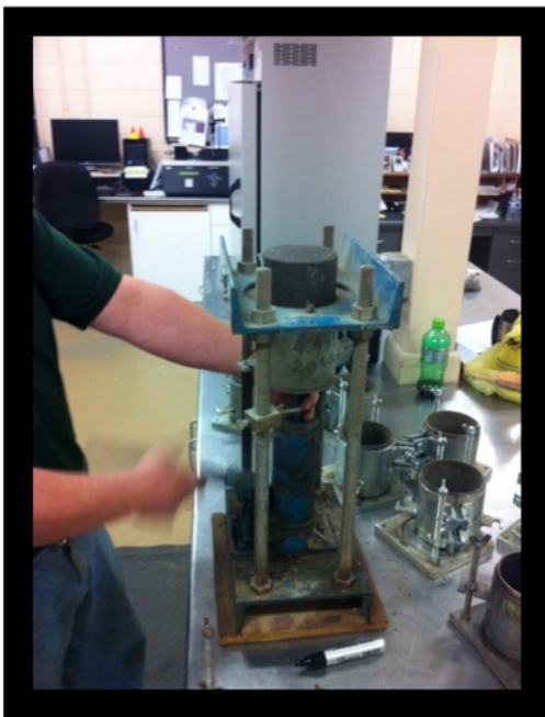
Figure 2.3 (Left): Picture of a cylinder getting removed from the mold Figure 2.4 (Right): Picture of cylinders submerged in water prior to compressive strength testing
