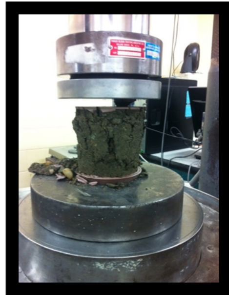
Figure 2.5 (Left): Picture of a cylinder prior to the compressive strength test. Figure 2.6 (Right): Picture of cylinder after the compressive strength test.
